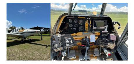
Airframe is eligible for upgrade to 10500 kit. Satloc Bantam, no flow control; CP Nozzles.
