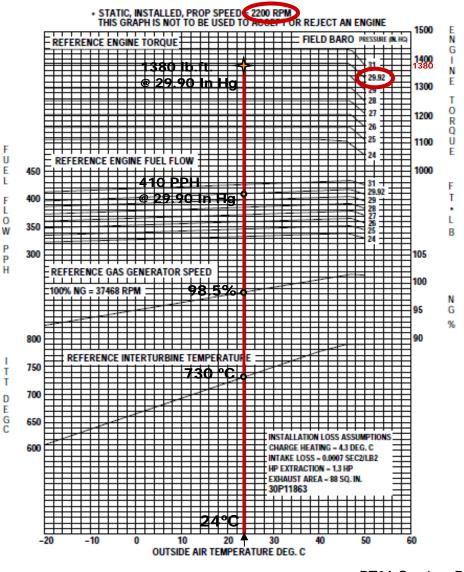
**Ground performance check** Record the OAT (°C) Record Field Barometric Pressure Close Air Bleeds Start the engine per POH Run at ground idle speed for 5 min Set propeller speed (Np - RPM) per chart Set Torque of the day per chart Stabilize for few minutes
