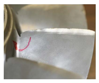
What cause the observed damage? Erosion due to sand / dirt ingested What can you do to improve your compressor performance?
